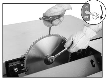
Figure 30. Installing the main blade.
